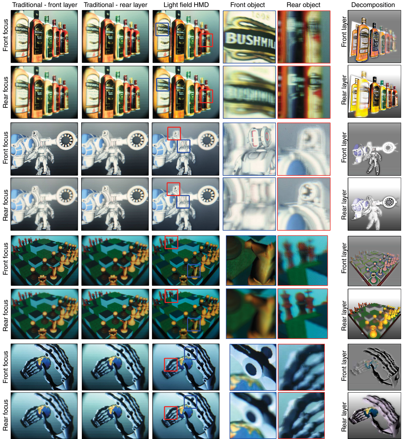
Figure S.3: We show a variety of computer-generated scenes photographed from one of our prototype light field stereoscopes. All results are generated with the proposed rank-1 light field factorization — factored patterns are shown in the right column. Retinal blur is clearly visible in all presented light fields. Slight moiree effects are barely visible to a human observer, but could be further mitigated using diffusers specifically engineered for this display configuration. The diffraction blur of the front panel limits the resolution observed on rear objects.
