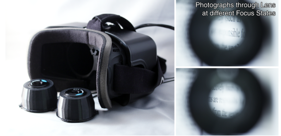
Figure 3. Photograph of HMD prototype and focus-tunable lens.
