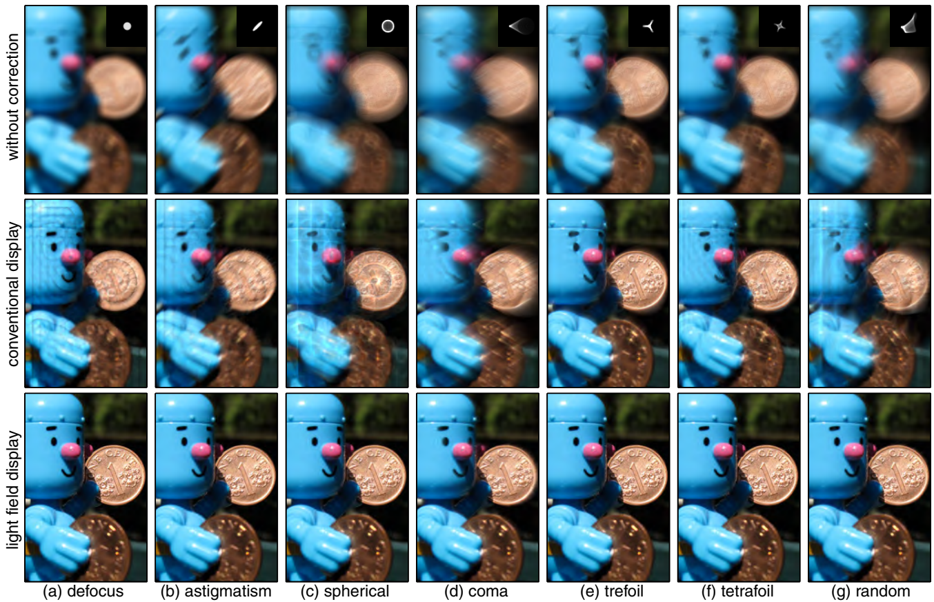
Figure S.7: Corrections for different aberrations. The lower order terms includes (a) defocus and (b) astigmatism, and the rest are all higher order terms.
