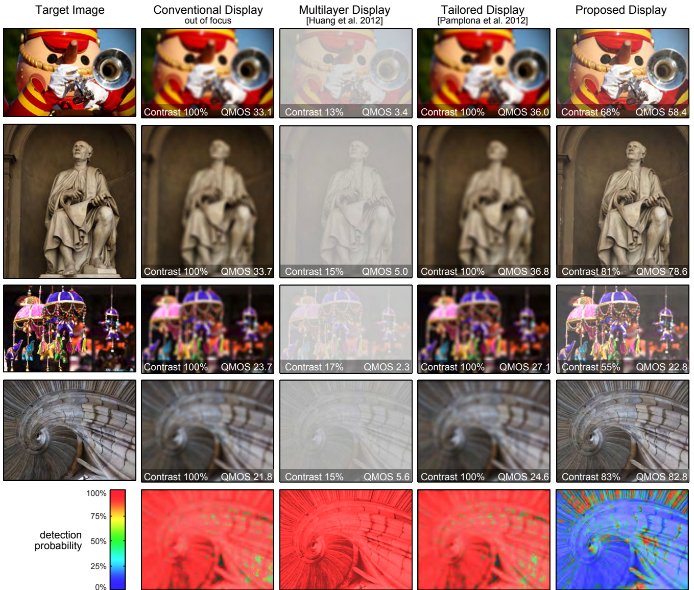
Figure 11: Evaluation and comparison to previous work. We compare simulations of conventional and vision-correcting image display qualitatively and quantitatively using contrast and quality-mean-opinion-square (QMOS) error metrics. A conventional out-of-focus display always appears blurred (second column). Multilayer displays with prefiltering improve image sharpness but at a much lower contrast (third column). Light field displays without prefiltering require high angular resolutions, hence provide a low spatial resolution (fourth column). The proposed method combines prefiltering and light field display to optimize image contrast and sharpness (right column). The QMOS error metric is a perceptually linear metric, predicting perceived quality for a human observer. We also plot maps that illustrate the probability of an observer detecting the difference of a displayed image to the target image (bottom row). Our method performs best in most cases. (Source images courtesy of Jameziecakes (flickr), Kar Han Tan, Mostaque Chowdhury (flickr), and Thomas Quine (flickr))
