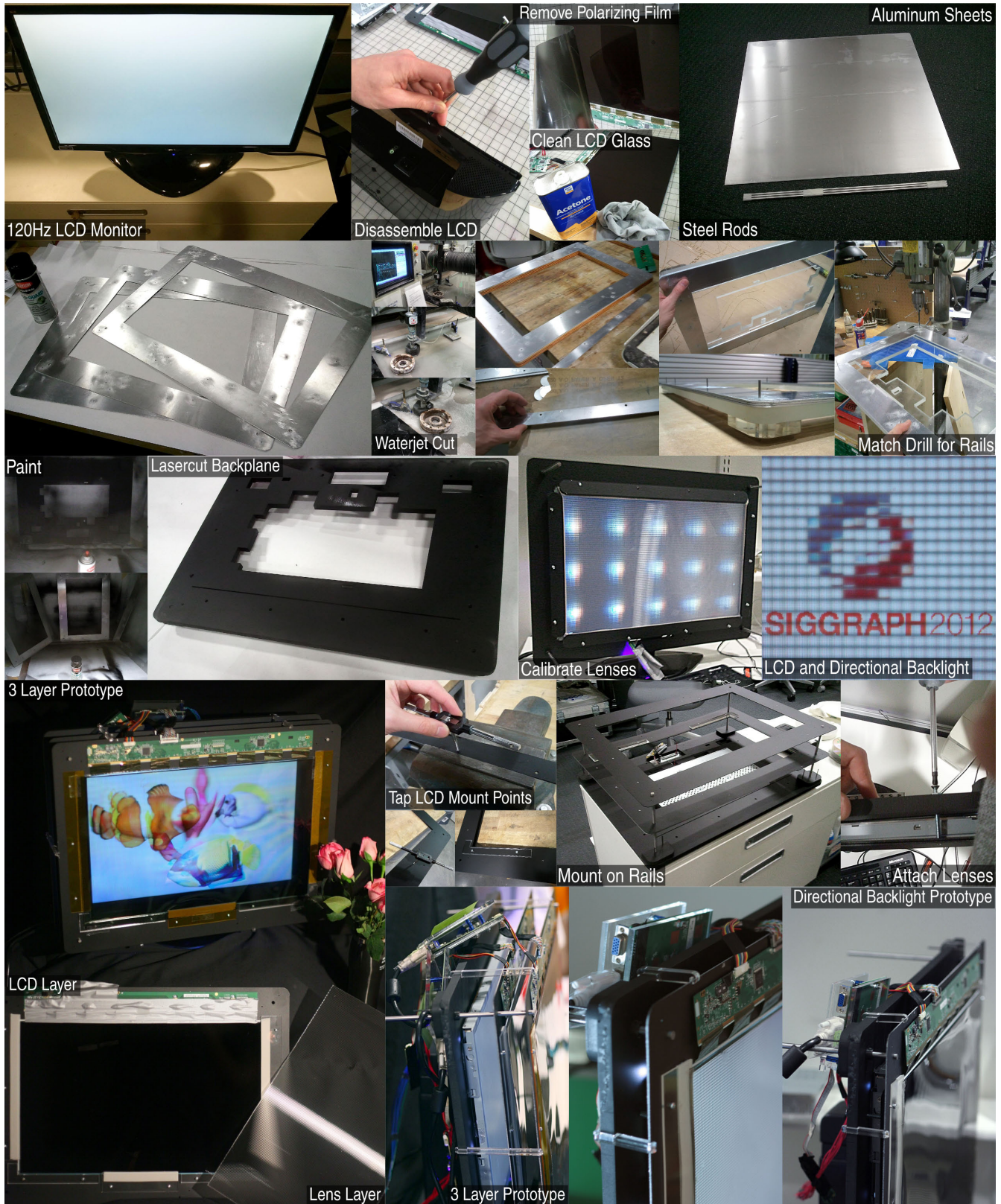
Figure S.11: Prototype construction. Three LCD panels were modified to implement two-layer and three-layer tensor displays. Custom waterjet-cut and laser-cut parts ensured accurate alignment of the display components.
