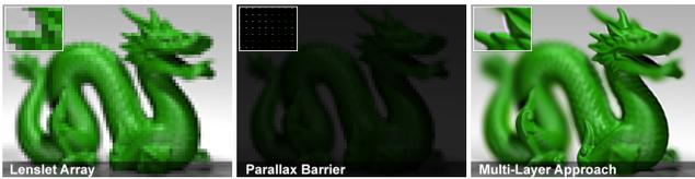
**Figure 13:** Benefits of multi-layer automultiscopic displays. Simulated views of the “dragon” are shown, from left to right, using integral imaging, parallax barriers, and our multi-layer approach. Display parameters are selected to allow  $7 \times 7$  views, leading to a similar reduction in resolution for conventional methods. Compared to parallax barriers, our approach is 49 times brighter and exceeds the resolution of both methods by a similar factor.
