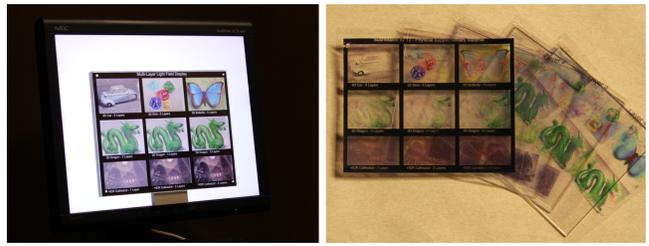
**Figure 2:** *Prototype multi-layer display. (Left) We fabricate a multi-layer display by separating transparencies with acrylic sheets and back-illuminating with a light box (e.g., an LCD panel). (Right) Printed transparencies and acrylic layers.*
