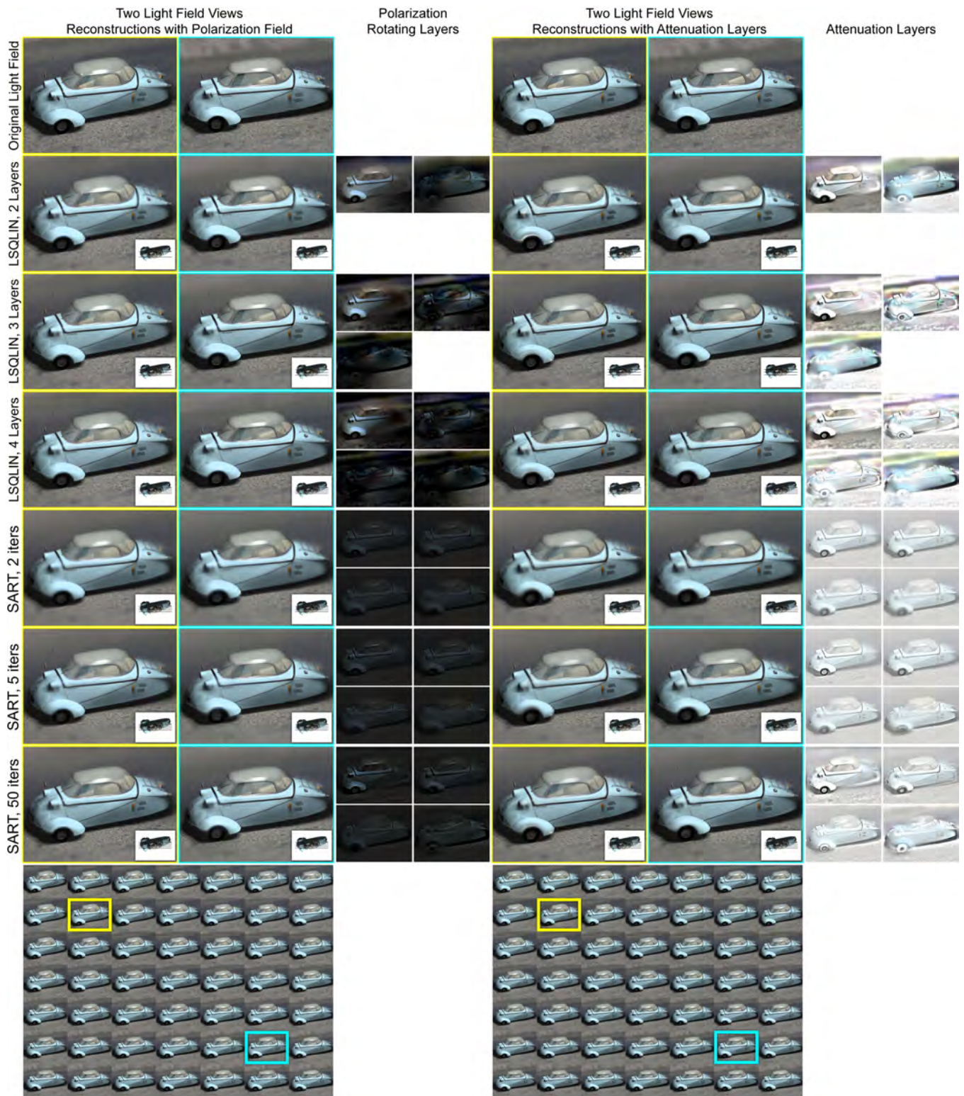
Figure S.5: Additional results for the “car” scene, taken from the archive available at http://www.layered3d.com . The display dimensions and optimization parameters match that of the prototype and correspond with those used in Figure S.2. The light field has a resolution of 512 \times 384 spatial samples and 7 \times 7 angular samples. The target imagery spans a field of view of 10 degrees.
