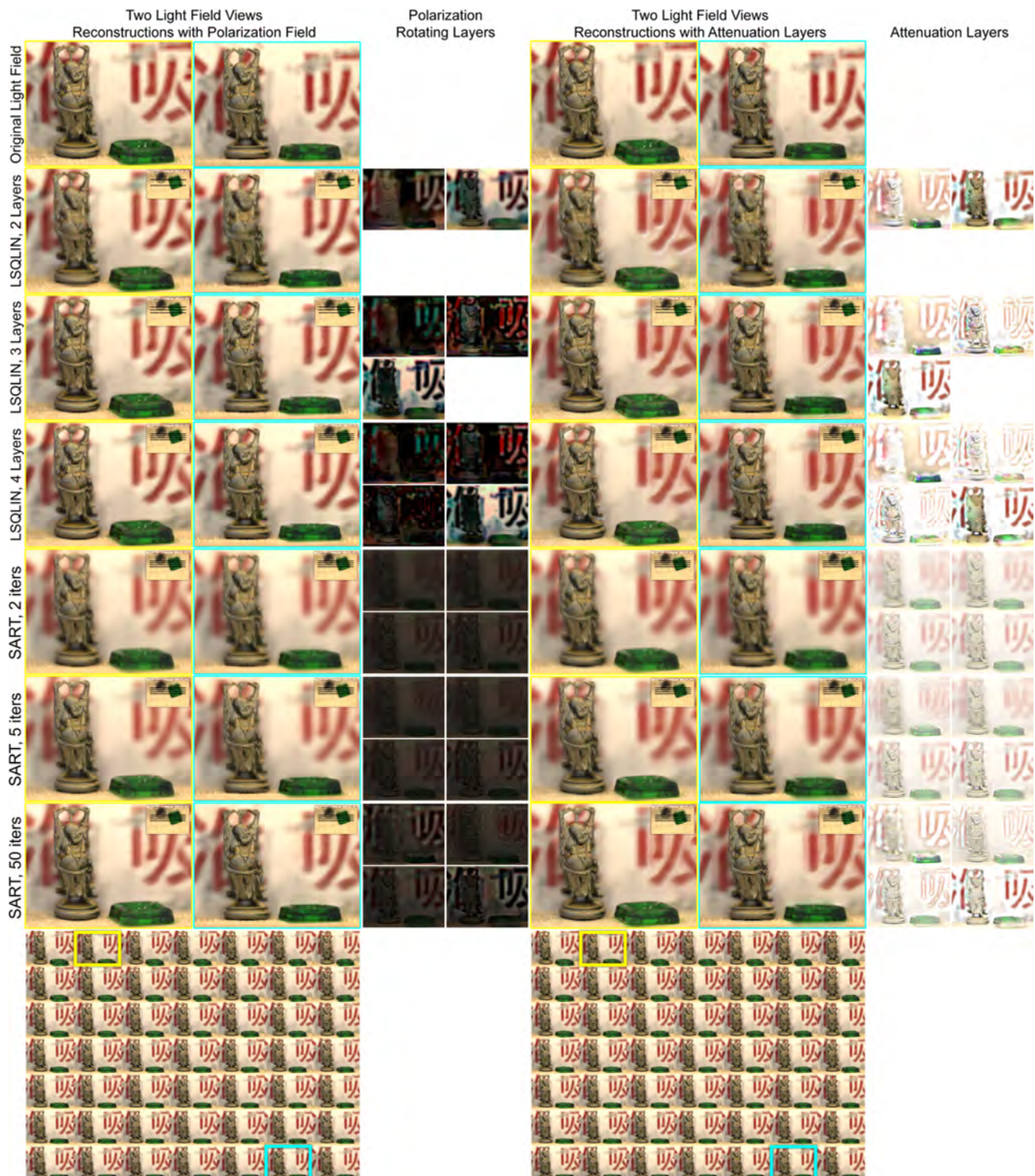
Figure S.2: Additional results for the “Buddha” scene, using the “Buddha” model from http://graphics.stanford.edu/data/3Dscanrep/ . Simulated views are compared for polarization-rotating layers (first and second columns) and attenuating layers (fourth and fifth columns). Rows illustrate, from top to bottom: target views, reconstructions using the off-line solver for two, three, and four layers (for the same depth range), and SART reconstructions with two, five, and fifty iterations with four layers. Columns three and six present decomposed layers.
