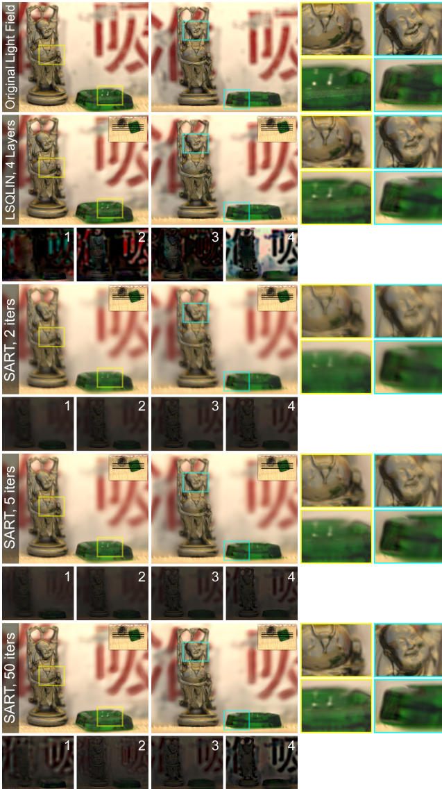
Figure 4: GPU-based SART allows real-time multi-layer optimization approaching the fidelity of the off-line solver. The first and second columns show different target views. Polarization-rotating layers are shown below each example. The off-line reference solver [Coleman and Li 1996] produces sharp reconstructions (second row). A small number of SART iterations causes blurring (third row). Additional iterations converge to the reference (bottom row), with five iterations yielding similar quality (fourth row). Note that simulated views are shown, rather than prototype results.
