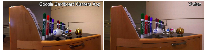
Fig. 15. Comparison between Google Cardboard Camera App and Vortex. The Cardboard approach exhibits strong vertical distortion for nearby objects and suffers from failure cases common to optical flow algorithms. Cardboard also requires the camera to be rotated on a much larger radius than Vortex, resulting in blurring of nearby content, e.g. as seen in the white teapot.
