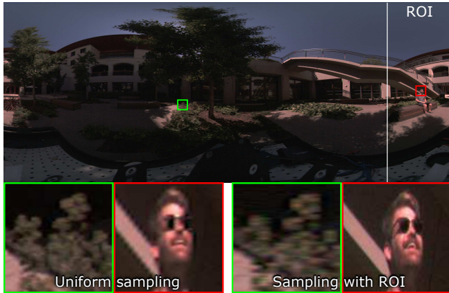
Fig. 16. Spatial nonuniform sampling: the ROI is sampled at an increased rate, and the rest of the scene at a decreased rate, yielding higher perceptual quality for the same total bandwidth. Here the ROI is sampled 8 times more densely than the rest of the scene.
