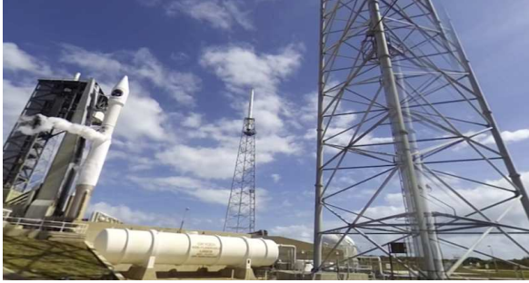
Fig. 5. A frame from a recent live broadcast 360° video, showing ghosting at the seam between camera FOVs. Stitching imagery from multiple cameras is inherently depth-dependent, making it difficult to perform well in real-time.
