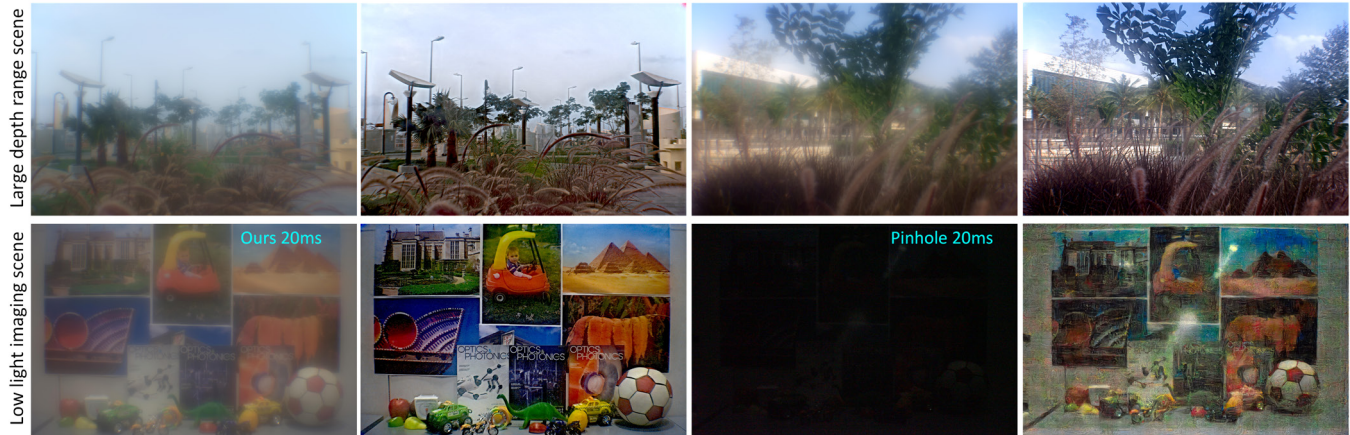
Fig. 12. Experimental results of large depth range imaging (top row) and low-light imaging (bottom row). The exposure time and ISO for the top two examples are set (3.125, 1) ms and ISO 50, while that for the bottom two examples are set (10 ms with ISO 500) and (20 ms with ISO 25,600).
