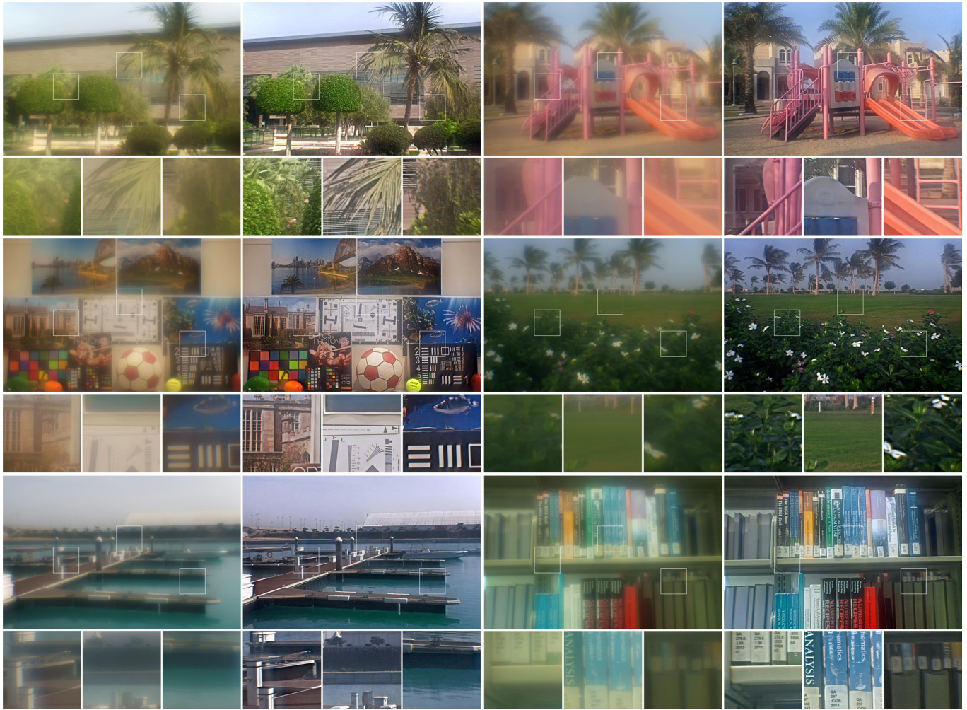
Fig. 11. Experimental results of dual-surface lens design (first two rows) and that of single surface lens design (third row) on real world scenes. For each pair, we show the degraded measurement and the reconstruction result. The exposure time for these images are set 0.8, 125, 0.5, 1.25, 0.5, 0.4 ms with ISO 50. Refer to supplementary document for more real world results.
