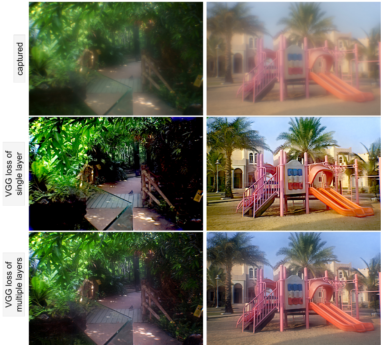
Fig. 11. Comparison results reconstructed using our network but with different settings regarding perceptual loss functions.
