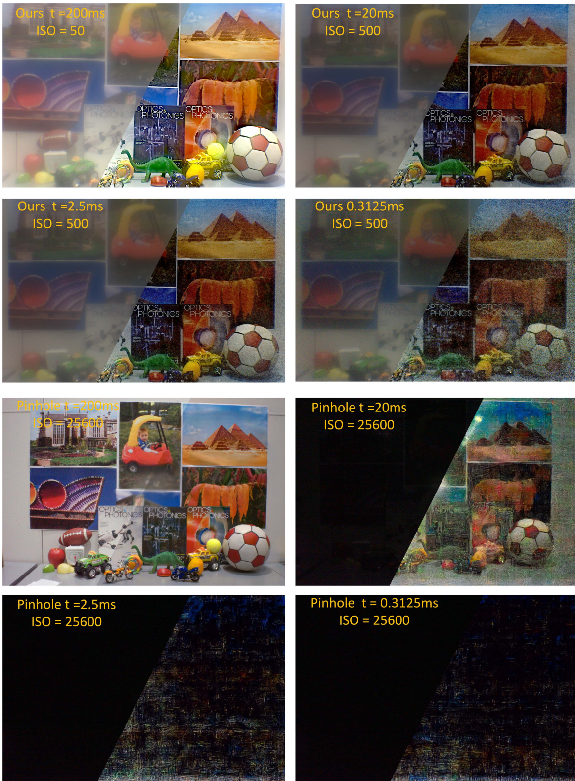
Fig. 12. Additional comparison results captured by our lens and a pinhole for low light imaging scenarios. For each example we present the exposure time and ISO for readers' information.
