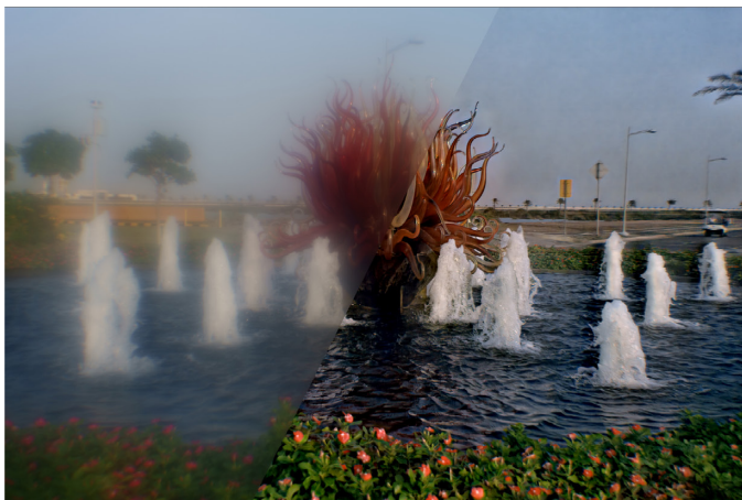
Fig. 8. Comparison results of our prototype lenses (left) and the SONY FE 1.4/50 lens (right) with a slightly different field of view due to the deviation of focal lengths. We show both measurement and reconstruction of ours side-by-side. With this numerical aperture, the SONY lens shows noticeable depth-dependent defocus effect. Note, our lens is a single element thin plate while the counterpart lens has an optical stack of more than a dozen of optical elements.
