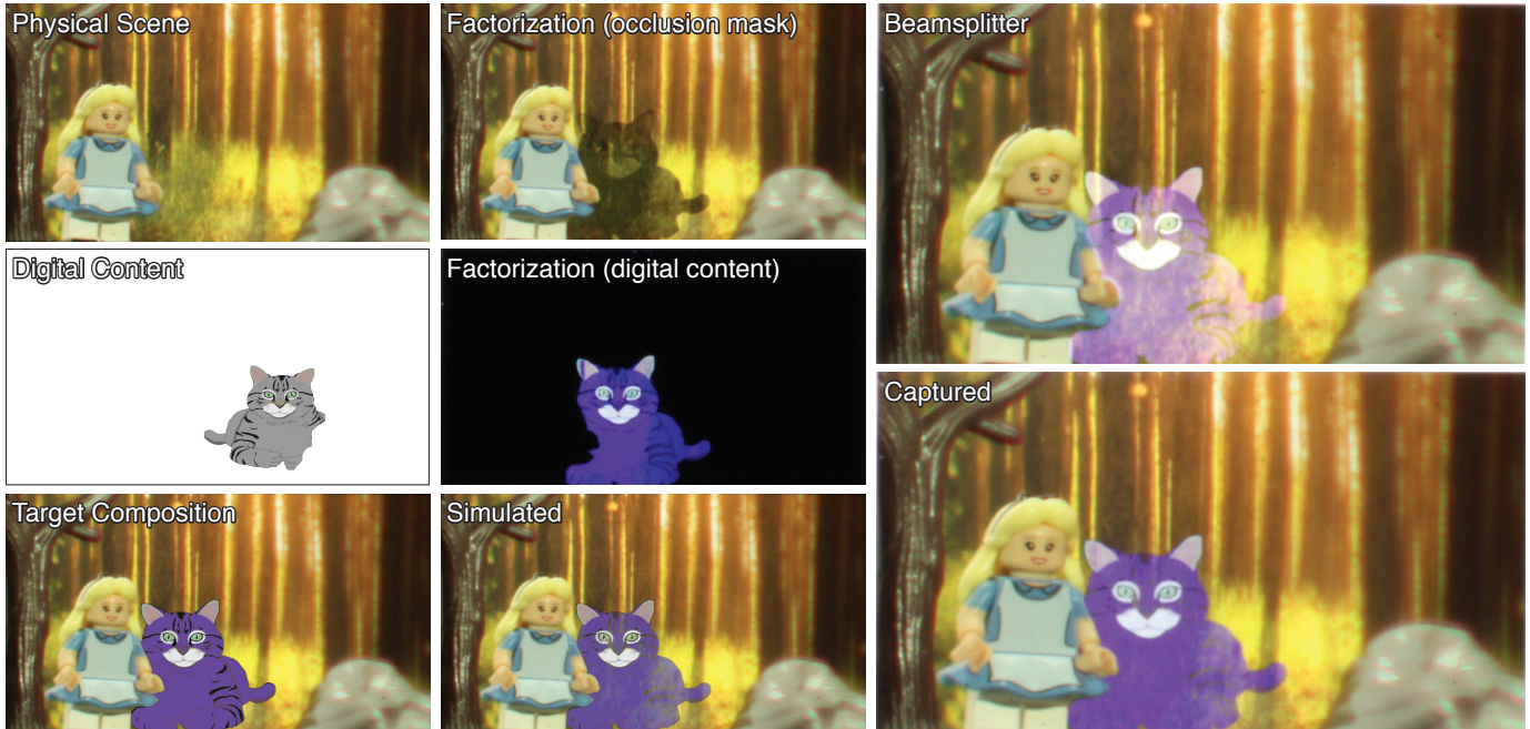
Fig. S.8. Purple cat scene . We combine a physical scene (left, top) and digital image (left, middle) to create a target composition (left, bottom). Our optimization-based approach then factors this into occlusion mask (center, top) and digital content (center, middle) components that combine to form a best approximation, as shown in simulation (center, bottom). This corresponds closely to the composition captured by our benchtop implementation (right, bottom), which shows significant improvement in color fidelity and light-blocking ability over a conventional beamsplitter approach (right, top).
