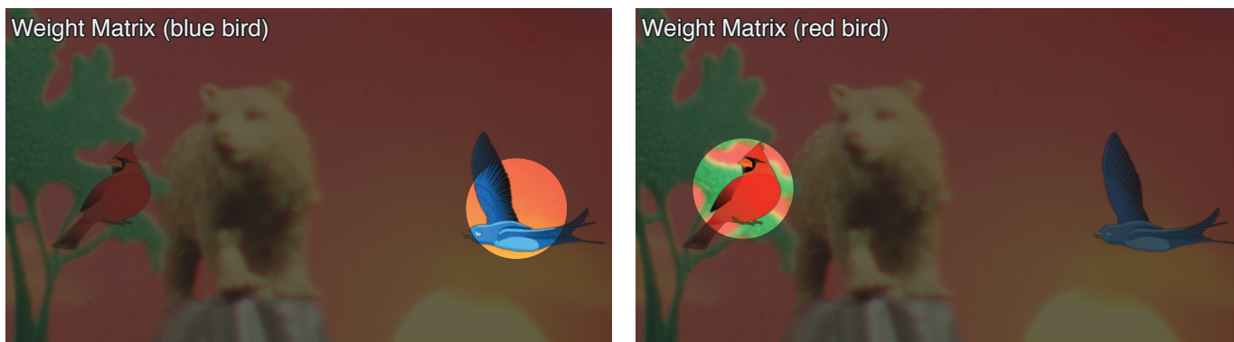
Fig. S.6. Bird scene weight matrix representation for blue bird (left) and red bird (right) gaze directions. Regions of faded image intensity indicate pixels given a weighting of 0.01, while the circular regions in full color indicate pixels given a weighting of 1. Each circular region has a diameter of 100 pixels, with the full image having pixel dimensions of 380 \times 680 .
